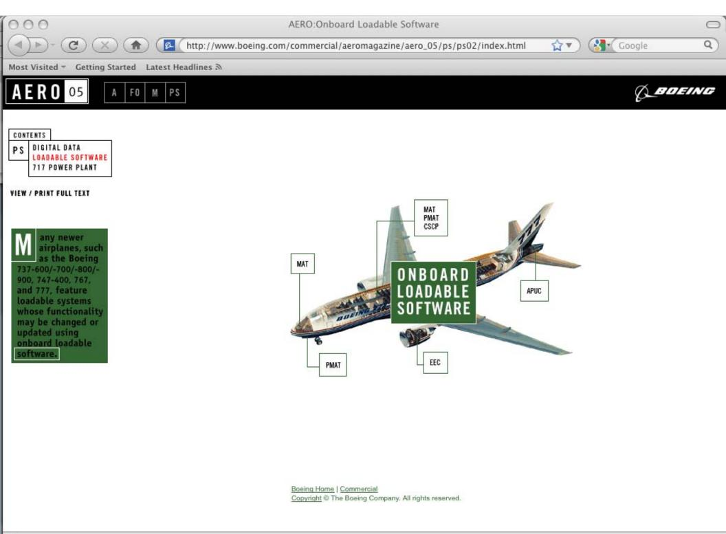
Many newer airplanes, such as the Boeing 737-600/-700/-800/-900, 747-400, 767, and 777, feature loadable systems whose functionality may be changed or updated using onboard loadable software. Modifying system functionality with new software instead of with modified or new hardware can help operators reduce the total number of hardware line replaceable units (LRU) in inventory, increase hardware commonality, and reduce airplane modification time.
